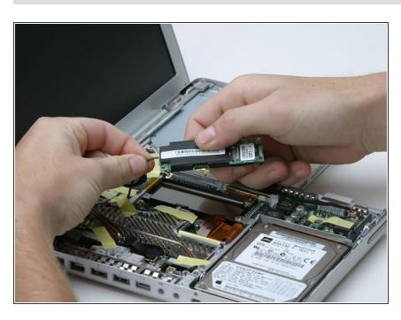
Disconnect the modem cable from the modem.
