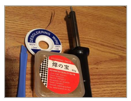
The materials needed for this are a solder gun, soldering paste and desoldering wire, also known as a wick.
