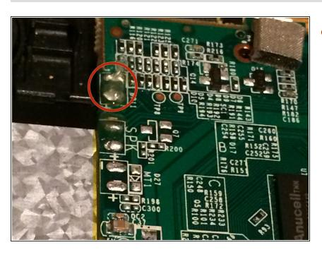
The location I will be de-soldering is right above the SPK location in the photo.
