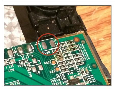
What's left over is clean points on the solder board, ready for fresh solder.
