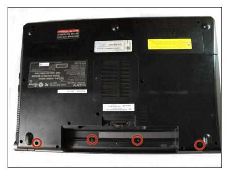
Remove the screws and flip it back.
