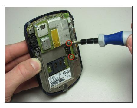
Remove the two T6 screws.
