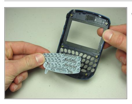
Remove keypad from front cover and replace or fix existing pad.
