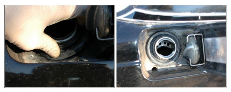
Use your thumb to press the new seal in around the filler neck. The new seal has a lip on the back that must be pressed in to the hole around the neck. This lip will grip the metal edge of the hole for a tight seal.
