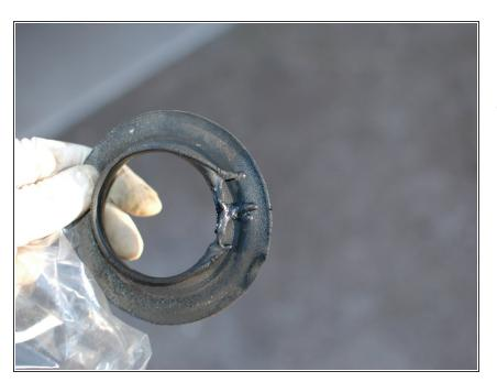
Here's one last look at the damage done by the biodiesel. The owner of this W123 will be more careful in the future not to drip fuel on the filler neck seal when filling with B99; at that concentration, biodiesel is very caustic to rubber. Lesson learned!
