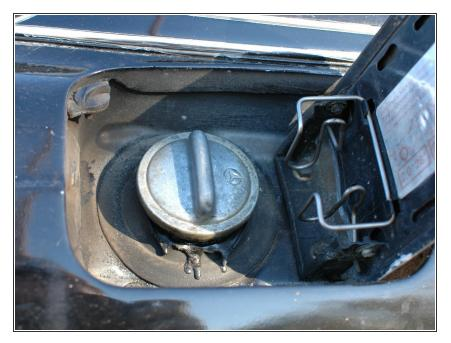
When inspecting your fuel filler neck seal look for dryness, brittleness, or like on this particular diesel W123 obvious damage. This was caused by drips of B99 biodiesel on the already aged rubber seal.
