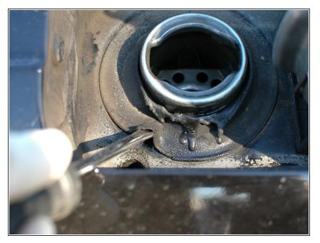
Gently pry around the edge of the old seal with a flat blade screwdriver or a large plastic spudger type tool. The old seals often stick slightly to the car.
