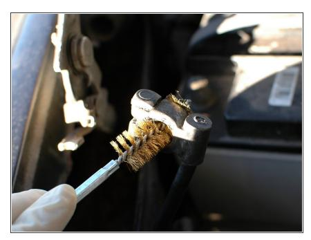
Use a soft metal brush, like the brass brush shown, to clean any corrosion off of the inside of the terminal. Follow this up with a spray of electric contact cleaner.
