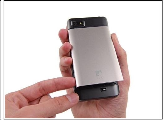
**i** There is a small indentation in the side of the phone near the bottom of the back cover.
