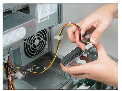
Remove the multicolored cable by grasping the plastic connector on either side and pulling with substantial force.
