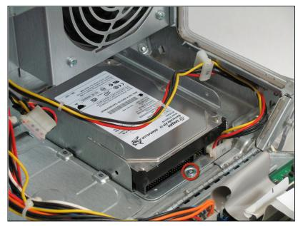
Remove the screw holding the hard drive to the computer.
