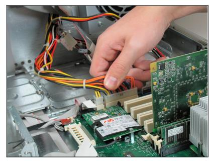
Disconnect the power supply cables from the mother board by pressing in the tab on the back of the connector as shown.
