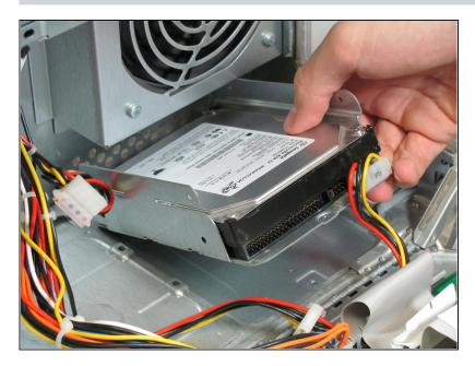
Pull the drive up and out of the computer.
