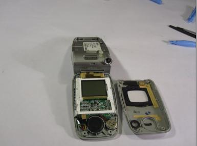
Remove plastic screen panel to reveal the internal components.
