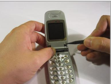
Remove the four rubber stoppers around the main screen using the pointed end of the spudger.
