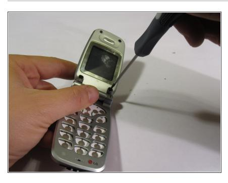
Use the Phillips #00 screwdriver to remove the four screws that were under the rubber stoppers.
