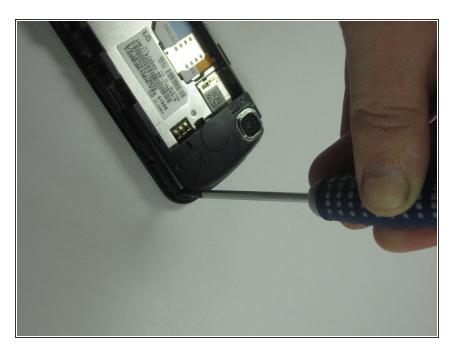
Remove the six screws around the outside of the phone using a Phillips #0 screwdriver.
