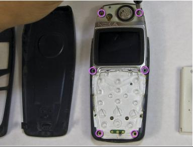
Remove the six screws around the front of the phone body with a T6 screwdriver.
