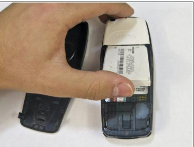
Lift the battery near the bottom and pry up.
