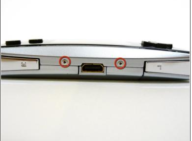
Remove the two tri-wing screws on the top of the Game Boy and the two screws next to the volume/contrast switch.
