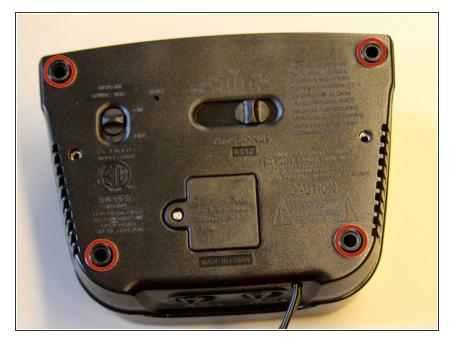
• Flip device upside down and remove the 4 foam pads at each corner.
