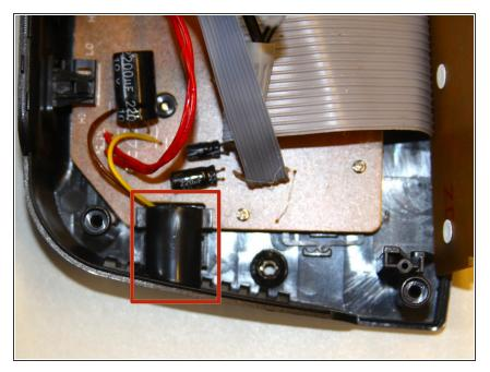
• Use the tweezers to slightly lift the circuit board, allowing the cylindrical alarm piece to slide out.
