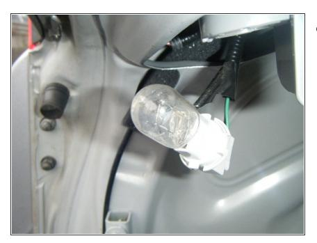
Remove bulb from tail light assembly.
