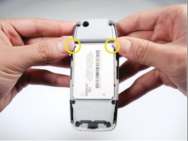
To release the battery, press the two tabs that are located directly above the battery towards the top of the phone at the same time.
