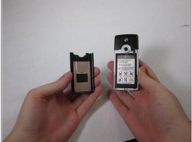
Slide the protective panel on the backside of the phone downward and remove it entirely, revealing the battery underneath.
