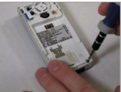
Remove the four screws located at each corner of the device.
