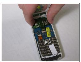
To place a new screen, slide the green ribbon connector into the ribbon clamp that the defective screen was pulled from.
