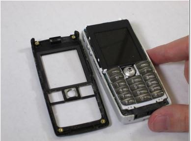
Gently lift and remove the front panel of the phone after removing the screws.
