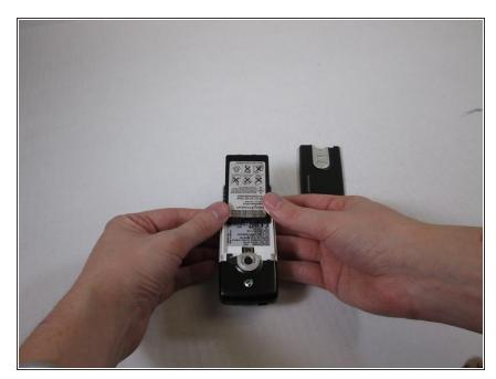
Slide the battery upward to remove.
