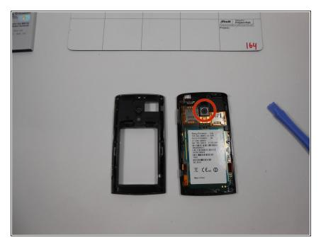
Once the clips are undone the back casing should dislocate and reveal the internal components of the phone. Camera location is identified on the image.
