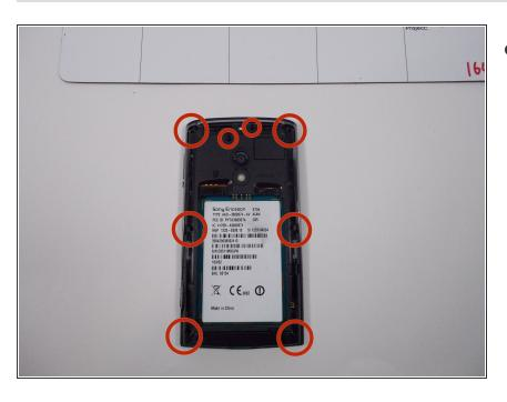
Remove eight 5mm screws as shown in the image. Use a T-6 bit.
