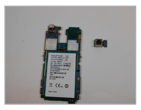
Once camera is removed, insert new functional camera part and reassemble
