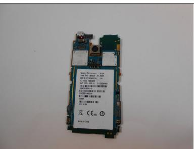
Once the interior casing is removed, dislocate the hardware by unlatching clip at shown location.
