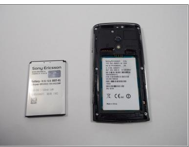
To access the internal components, such as the camera, we need to flip the phone with the screen facing down. Once this is done remove the battery.
