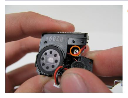
Unscrew one Phillips screw, using a #0 Phillips screwdriver.
