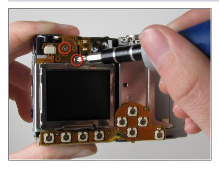
Unscrew two Phillips screws above the LCD using a #0 Phillips screwdriver.
