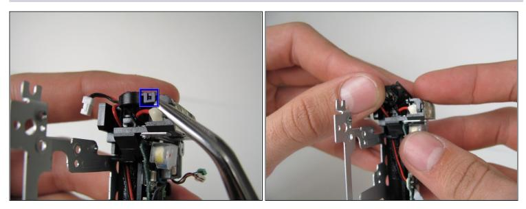
• Lift off the tab on top of flash assembly.
