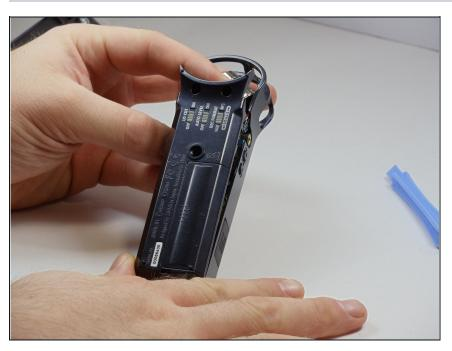
Carefully pry up the top end of the back cover using one finger.
