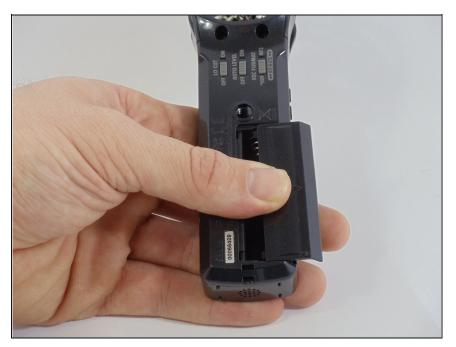
Remove the battery cover, pressing down on the tabs and sliding.
