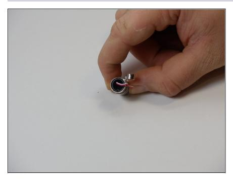
Insert the leads of the new microphone into the plastic insert and reinsert into the silver microphone casing.
