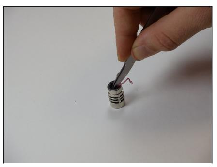
• Insert the tip of the angled tweezers into the hole in the black plastic located within the microphone case. Use the tweezers to pull the microphone out of the casing.
