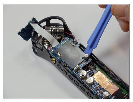
Use the plastic removal tool to gently pry up the blue circuit board, allowing access to the microphones.
