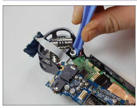
Use a plastic removal tool to pull the microphone casing off of its post.
