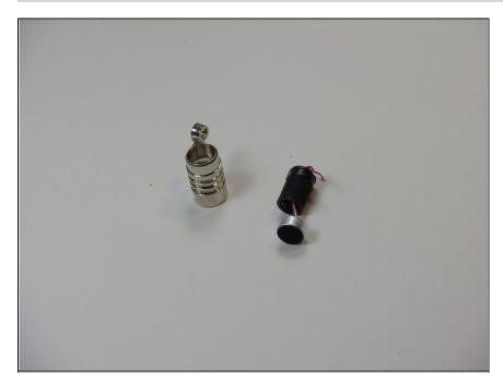
Remove the faulty microphone by pulling the leads through the black plastic insert.
