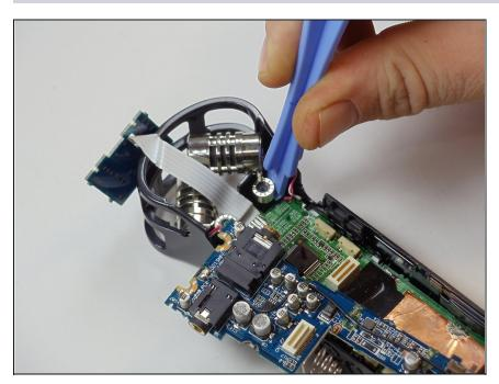
• Re-attach the microphone case to the post it came off of.
