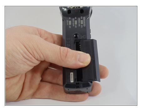
Remove the battery cover by pressing down on battery cover and sliding it to the right.
