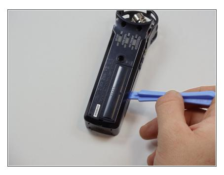
Remove the back cover (using a plastic removal tool around the edges if needed).
