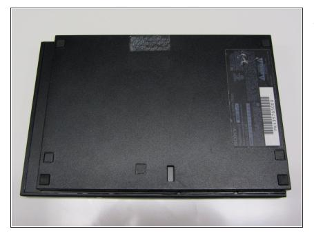
Disconnect all cables from the console and flip the unit over to reveal its base.
