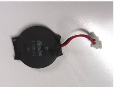
• Gently lift and remove the battery from its compartment using a spudger.
