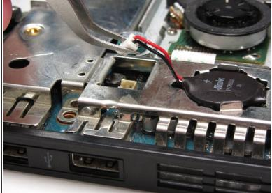
Lift the connector from the motherboard with a pair of tweezers using a firm, upward force.
