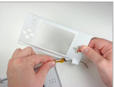
After opening it, carefully unhinge them from each other by sliding the bottom piece to the left and the top piece to the right.
