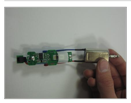
remove the inside on the razor which includes the chip set, battery, motor and switch.
