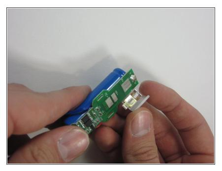
Remove the white piece. Be careful doing so because the chip set is delicate and breaking that would result in replacing that as well.
