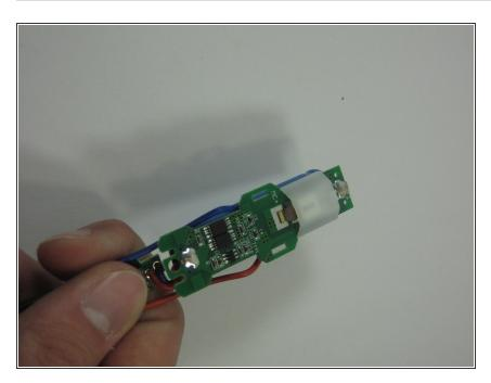
focus on the chip set and the white piece on top. The white piece is the switch that turns the razor on and off.
