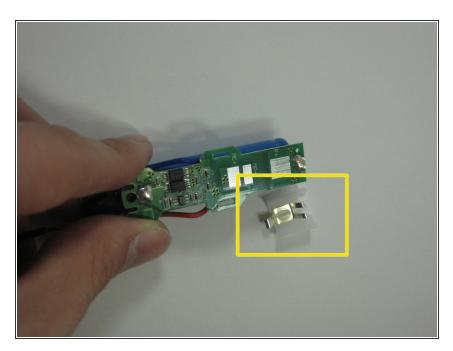
Upon removing the switch, exchange the broken part with the new one that you bought and replace it. Once installed put the razor back together and now you will be able to turn the razor on and off.
