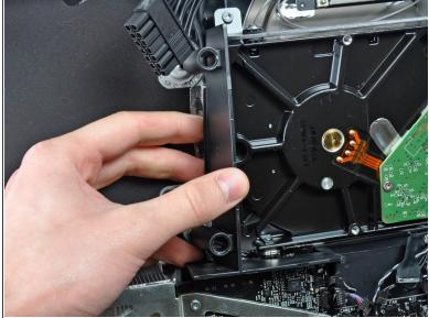
Remove the plastic ducts from the side of the LED driver board and the hard drive by pulling them away from the outer case.
