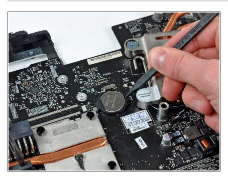
Use the tip of a spudger to pry the PRAM battery out of its socket on the logic board.
