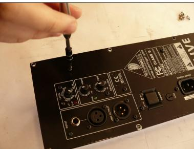
Remove the 4, 7/32" long machine screws with a #2 phillips head screwdriver.
