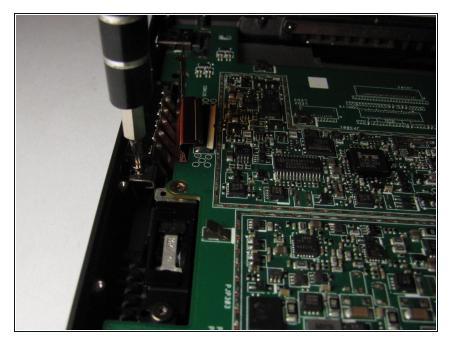
• Unscrew the two T5 torx screws located on each side of the charging port.
