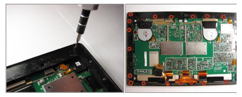
Using a T5 Torx screwdriver, unscrew a total number of 23 screws located on the outside panel of the Surface Pro.
