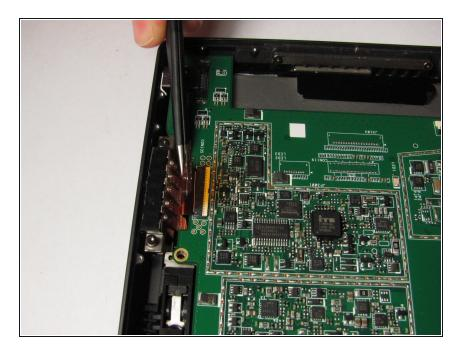
• Pull out the orange charging port strip using tweezers
