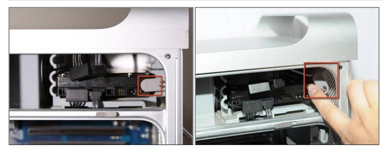
• Rotate up plastic tab labeled "B" on the right hand side of hard drive.
