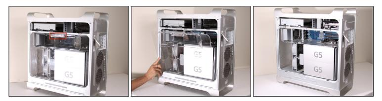
• Remove the air deflector (the clear plastic cover) by pulling on the handle.
