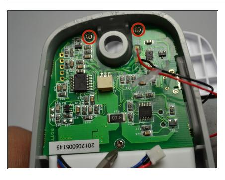
Unscrew the three 2mm screws holding the circuit board down using a Phillips #1 screwdriver.
