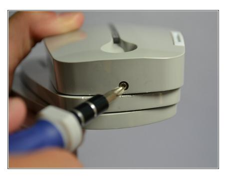
Using the Phillips #1 screwdriver, remove the 2mm screw located on the bottom of the device, near the hinge.
