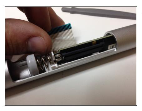
Keeping the connection cable, push out the logic board's placement
