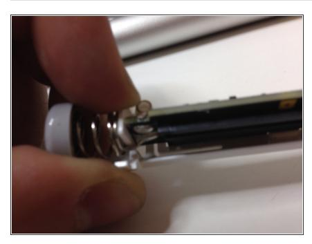
Unlock the latch of the logic board
