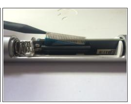
Pull the lock up and disconnect the connection cable
