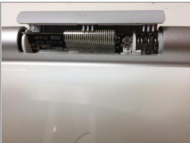
Insert a metal spudger to open the plastic part under the Keyboard
