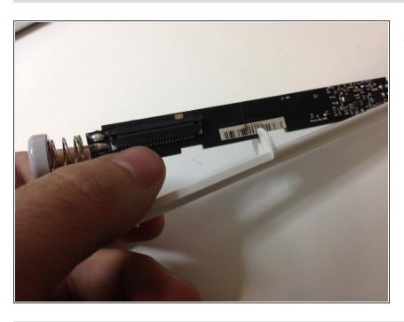
Remove the logic board from the placement
