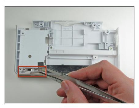
Carefully use a pair of tweezers to remove the volume switch.
