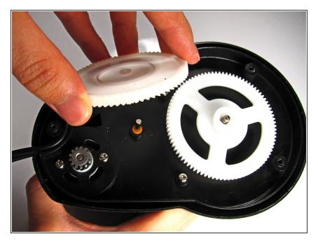
Remove the smaller white gear by lifting it up with your hand.
