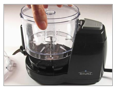
With your hand, twist the container counter-clockwise until it unlocks from the base. Remove the container by lifting it straight up.
