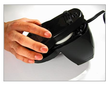
Firmly lift the bottom cover off of the base.
