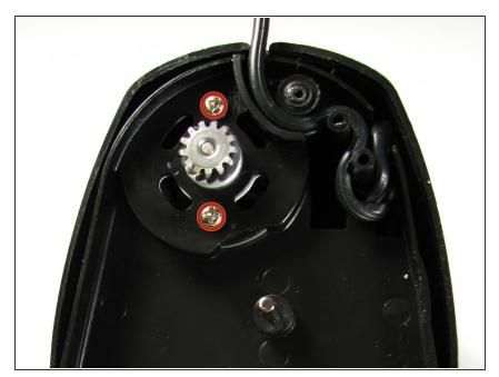
Use a Phillips #2 screwdriver to remove the screws that attach the motor to the base.
