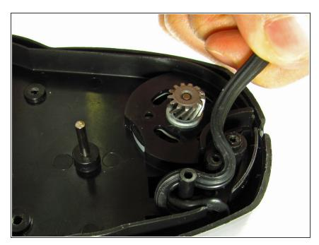
Unwind the power cord from the base pegs.
