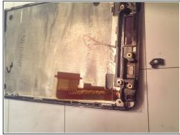
This plastic piece goes directly over the screw hole. It falls out easily, but when removing and replacing it only goes back in place in one direction. The shape of the plastic piece makes it go into place in only one direction.
