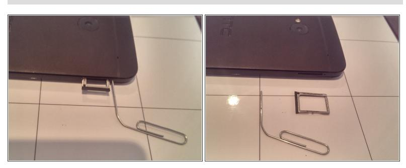
Remove the SIM card and tray by ejecting it with a paper clip or SIM Ejector Tool
