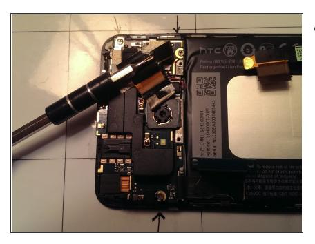
Remove the three screws using the Phillips #000 screwdriver as indicated in the photo
