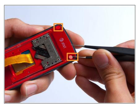
Remove the two red sticker screw coverings at the top corners with tweezers.
