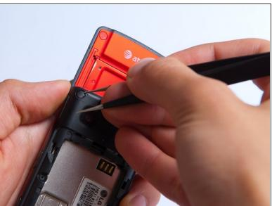
Remove the two screw covers at the top of phone with tweezers.
