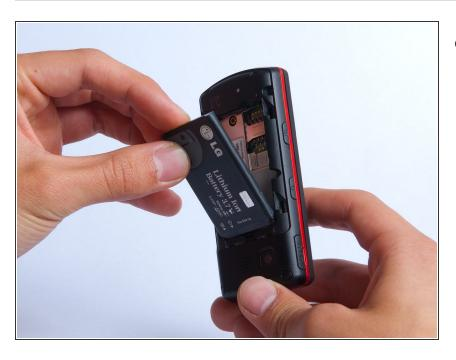
Lift and remove the battery.
