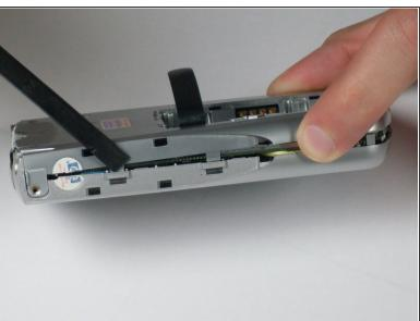
Remove the back faceplate by pushing and loosening the 4 side slots (2 on each side).
