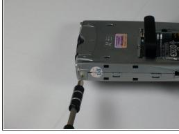
Using the T5 Torx screwdriver, remove all six screws on the back and all screws on each side of the device.
