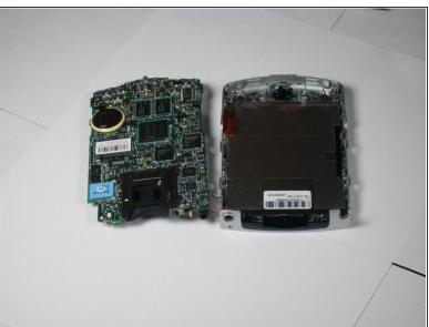
Press on side tabs to loosen and remove the LCD screen.
