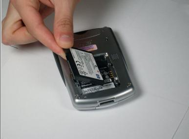
Pull on the black tab to lift the battery out of the battery compartment.
