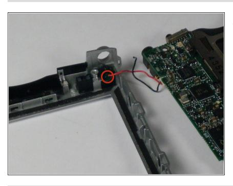
Remove the faceplate by unscrewing the green screw located on the top right of the front faceplate.
