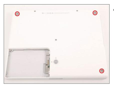
Remove the three newly-revealed Phillips screws.
