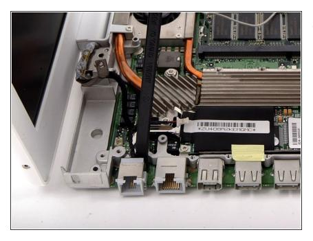
Wedge a spudger between the RJ-11 board and the metal framework and slide the board away from the logic board.
