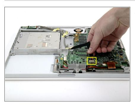
Disconnect the DC-In cable from the logic board.
