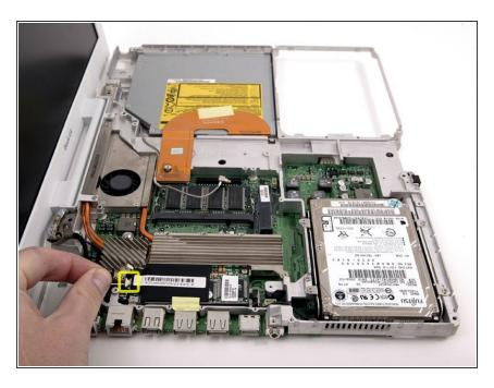
Disconnect the RJ-11 cable from the modem.
