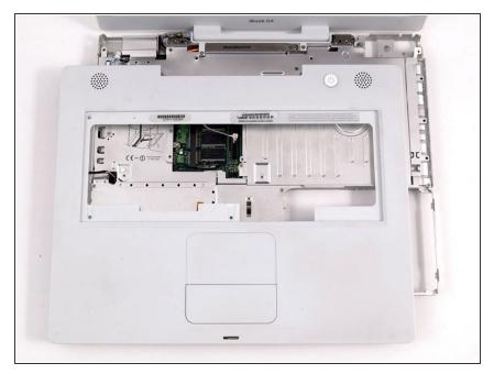
Carefully lift the upper case about half of an inch and move it so that you can access the power and speaker cables.
