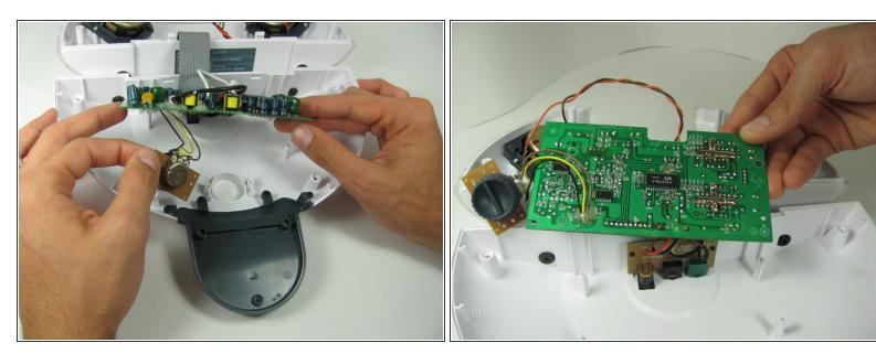
• Lift up on both the motherboard and brown circuit board that contains the light intensity dial and turn the motherboard over.
