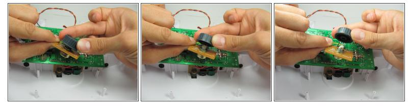
Hold the brown circuit board with one hand and the light intensity dial with two fingers of your other hand and carefully pull them apart.
