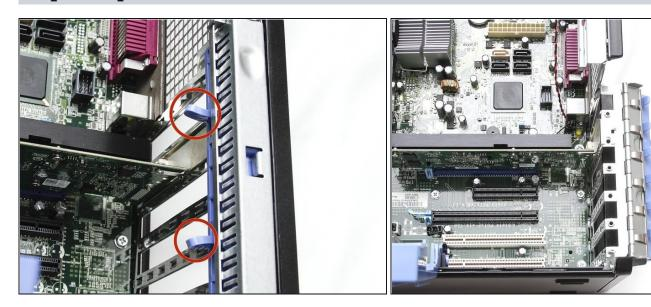
• Squeeze the two release tabs together and pivot the secure hatch to the right to open.
