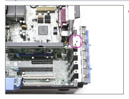
Hold the card by its top corner and metal bracket and pull it out of its slot.
