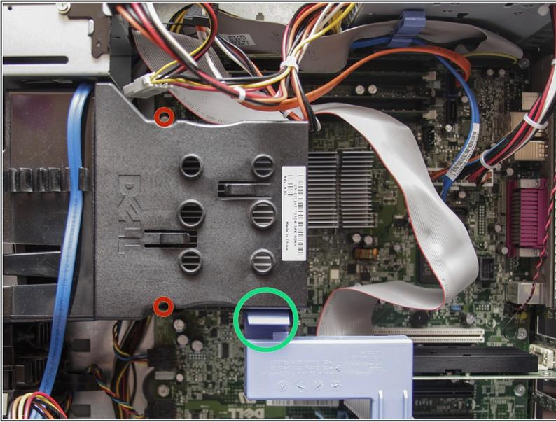
**⚠ CAUTION:** Even though the heat-sink assembly has a protective plastic covering, be careful when touching it -- the assembly may still be hot if your PC was just on.
