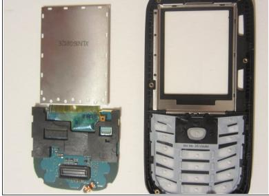
Use a tool to pry open the LCD display. Remove the display and the circuit board that it's connected to.
