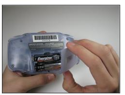
• Remove the back battery cover by pinching down on the tab and pulling outward.
