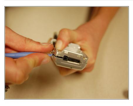
Use the plastic opening tool and slide it around the phone to pull apart the front and back casing.
