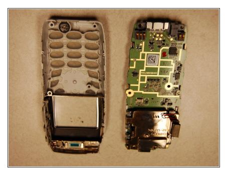
Use the plastic opening tool to remove the motherboard from the front case.
