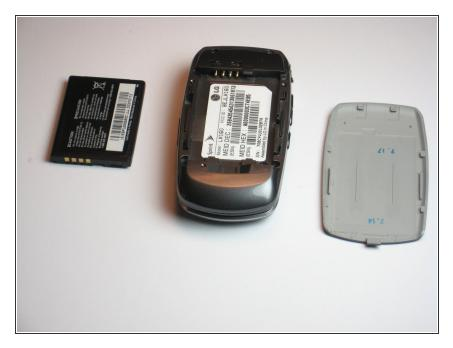
Remove the battery completely from the phone and place the battery off to the side.
