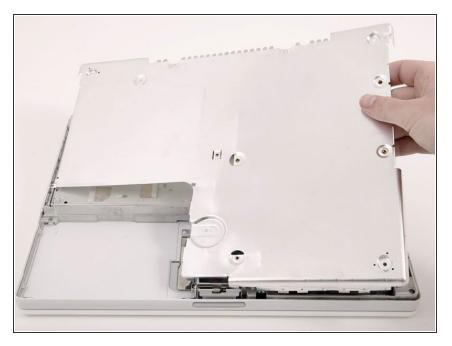
Lift the bottom shield off.
