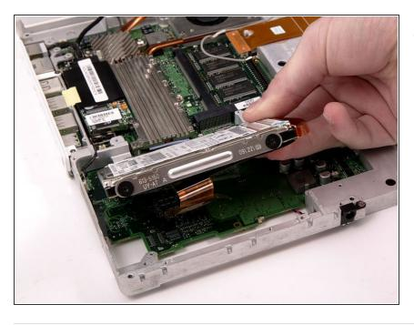
Lift the hard drive up, carefully guiding the cable through the slot in the lower case.
