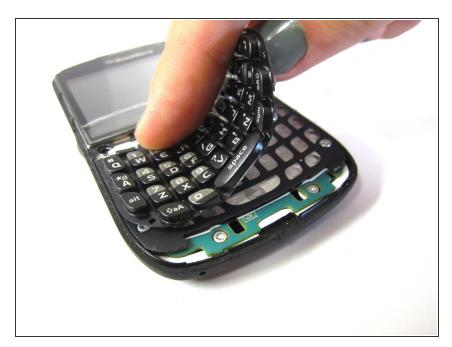
Lift and remove the keyboard.
