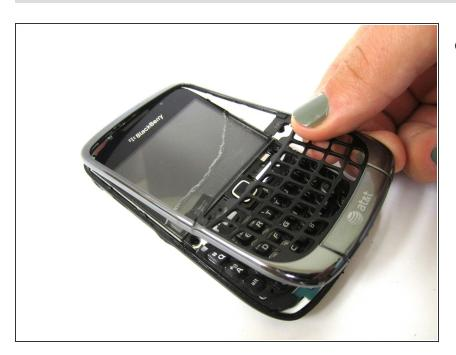
Lift and remove the frame.
