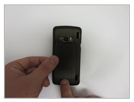
Slide the release latch down and toward you while lifting up on the left side of the battery cover.
