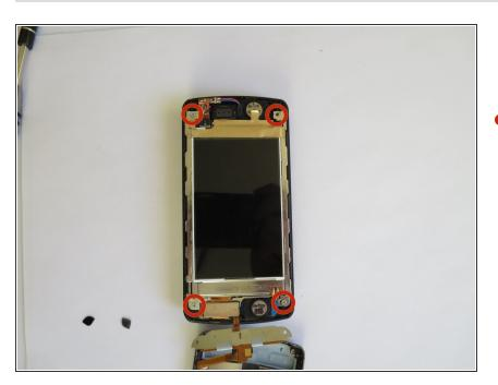
Remove the four 1.5mm #000 Phillips screws at each of the corners of the phone, using the Phillips #000 screwdriver.
