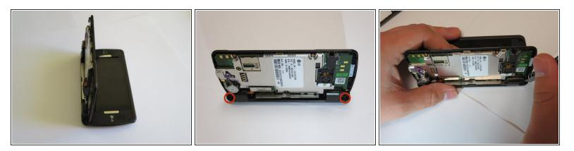
(i) Open the phone at a 90 degree angle. This needs to be done in order to reach the screws.
