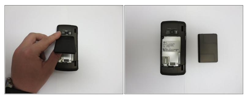
• Lift the edge of the battery to remove it.
