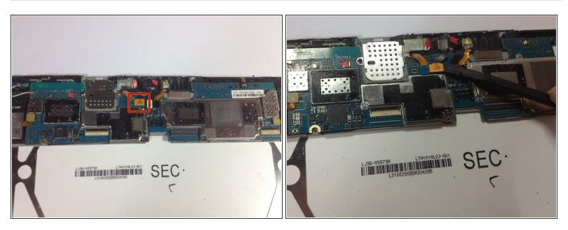
• Use the spudger to pry up on orange connection. This is the connection to the front facing camera.
