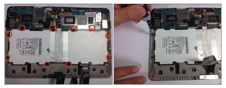
• Remove the ten 3 mm Phillips #00 screws surrounding the battery.
