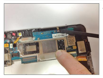
Hold down the motherboard with your finger and use a spudger to gently pry up the connection for the volume keys and power key.
