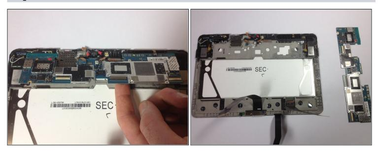
• Lifting from the bottom edge, gently remove the motherboard.
