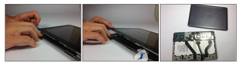
• Using the plastic opening tools, continue to carefully run along the right and bottom edge, and then lift the screen from the back panel.
