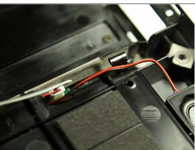
Locate the plug for the speaker wires on the bottom of the laptop.
