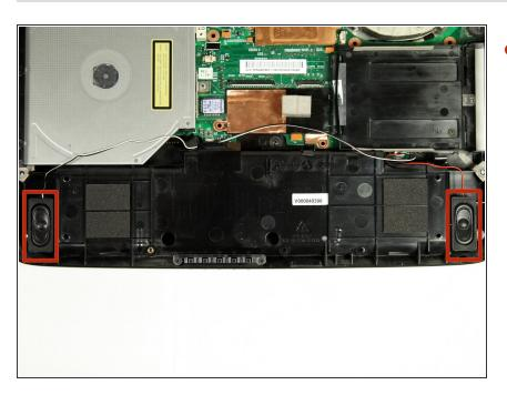
Remove the speakers by sliding them straight up. They should slide out with ease.
