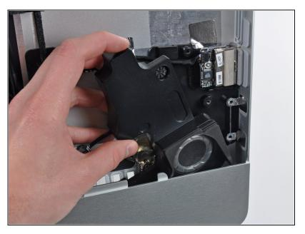
Gently lift the right speaker assembly out of the outer case.
