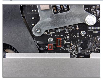
Disconnect the CPU fan and power button by pulling their connectors toward the left edge of the iMac.
