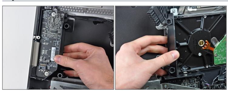
Remove the plastic ducts from the side of the LED driver board and the hard drive by pulling them away from the outer case.
