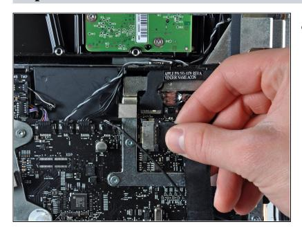
Disconnect the audio port cable by pulling its connector toward the right side of the iMac.
